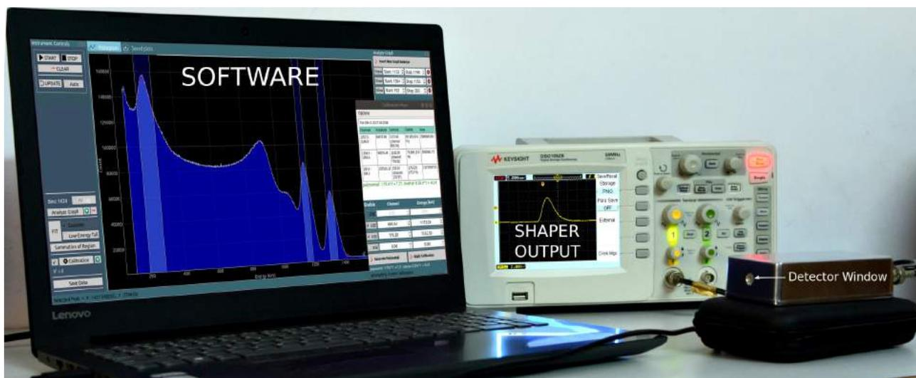
Figure 1: Gamma spectrometer
